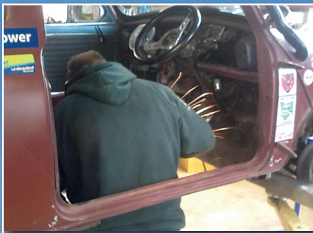
Matt Webb grinding the old floor.
