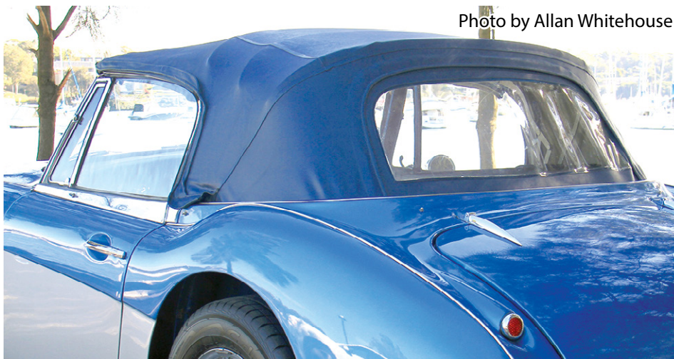
BJ7 was first Austin-Healey with wind-up windows and a truly easy to erect hood.
