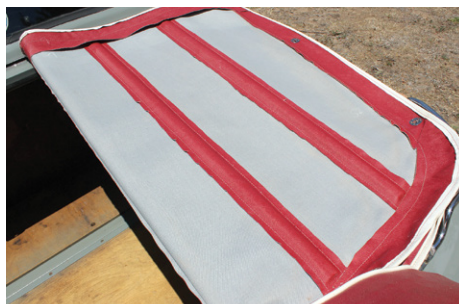
Timber strips sewn into tonneau.
