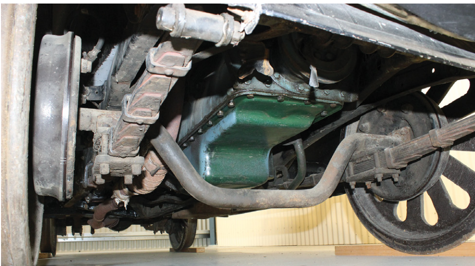
Front axle was narrowed and spring shackles moved inboard, with standard hubs used.
