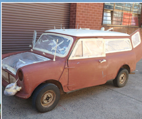
Stickers removed and ready to paint.
