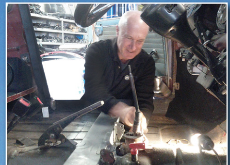
Craig Illing bolts in the seat brackets.
