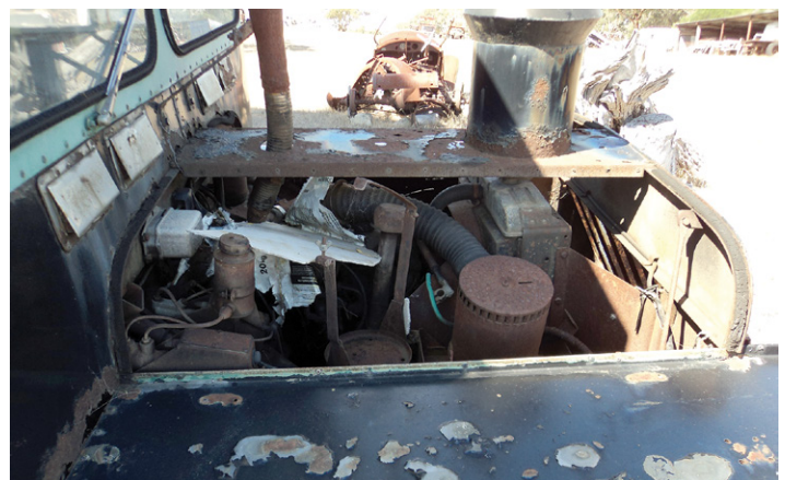
Engine was exposed to weather, has seized and is being replaced.
