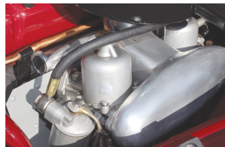
ZB's 1½" carbs helped lift engine to 68bhp.
