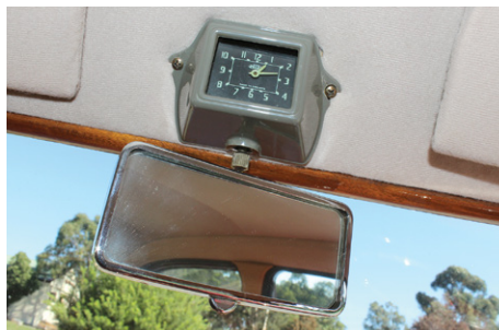
Anti-dazzle dipping mirror in all Z-series.
