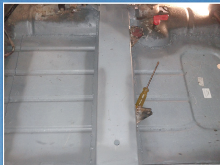
The new floor and cross member.
