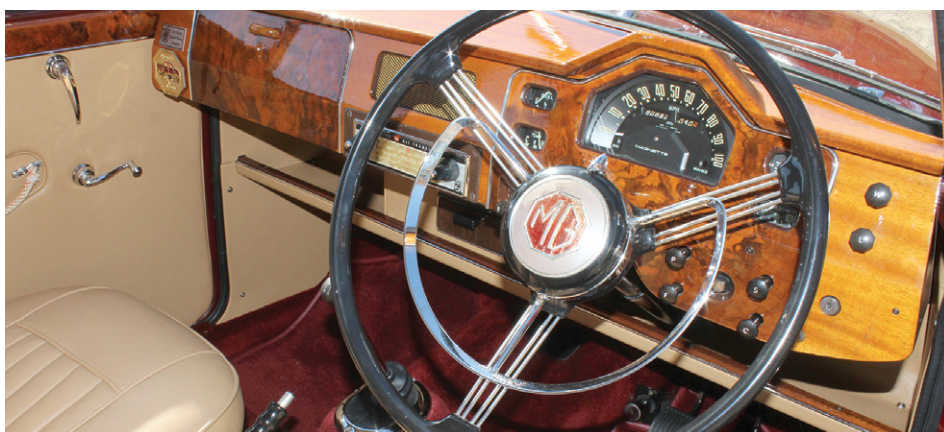
Slightly dished steering wheel and under-dash parcel shelf were features of the ZB.
